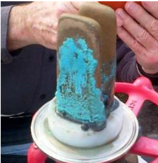
The anodes were inspected regularly and both anodes required regular monthly cleaning because of a build-up of blue scum which formed on each anode (Photo) This scum was soft and easily removed by scraping and washing with water.
